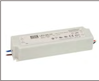
Type: Meanwell LPV Series Power: 20/35/60/100/150W Input Voltage: 100V-264V/AC Output Voltage: DC12/24V IP67 Waterproof
