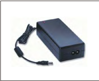
Type: LED Desktop Adapter Power: 36/48/60/72/96/120/150W Input Voltage: 100V-264V/AC Output Voltage: DC12/24V Chinese/American/European/Australian Plug available Non-waterproof
