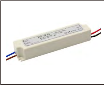
Type: Plastic housing Waterproof Power: 20/35/60/75/100W Input Voltage: 100V-264V/AC Output Voltage: DC12/24V IP67 Waterproof
