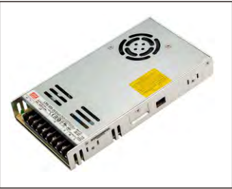
Type: Meanwell LRS Series Power: 35/75/100/200/450W Input Voltage: 100V-264V/AC Output Voltage: DC12/24V Non-waterpfoof
